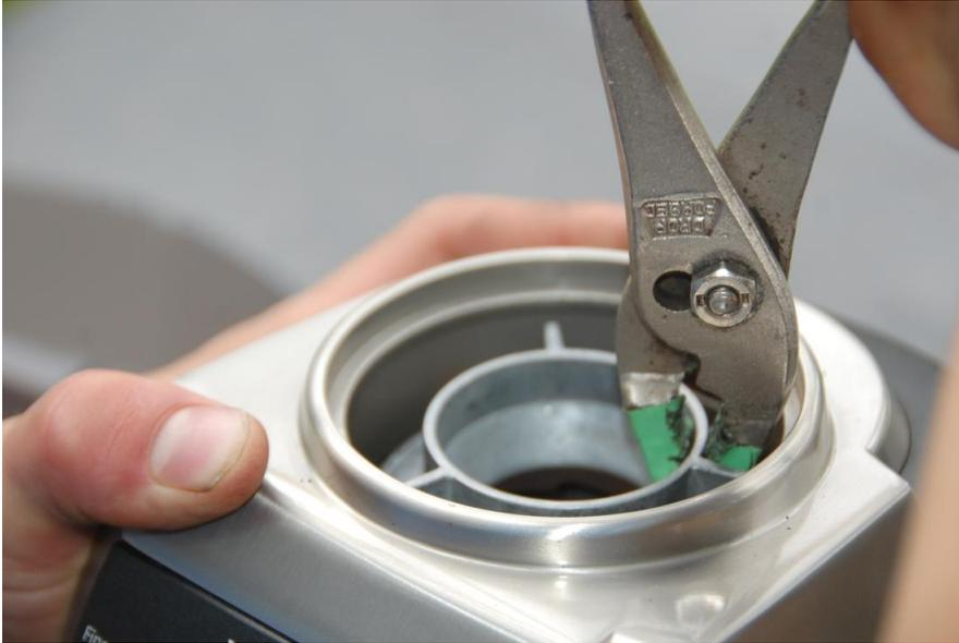
Remove the three flathead screws and separate the ceramic burr from the carrier.
