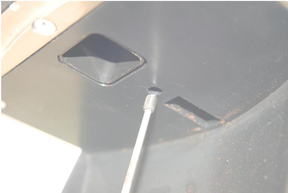
Loosen the 2.5MM Allen screw found in the rectangle slot. Moving the screw towards the front of the grinder (arrow pictured below) makes the grind coarser. Then tighten the 2.5mm screw.
