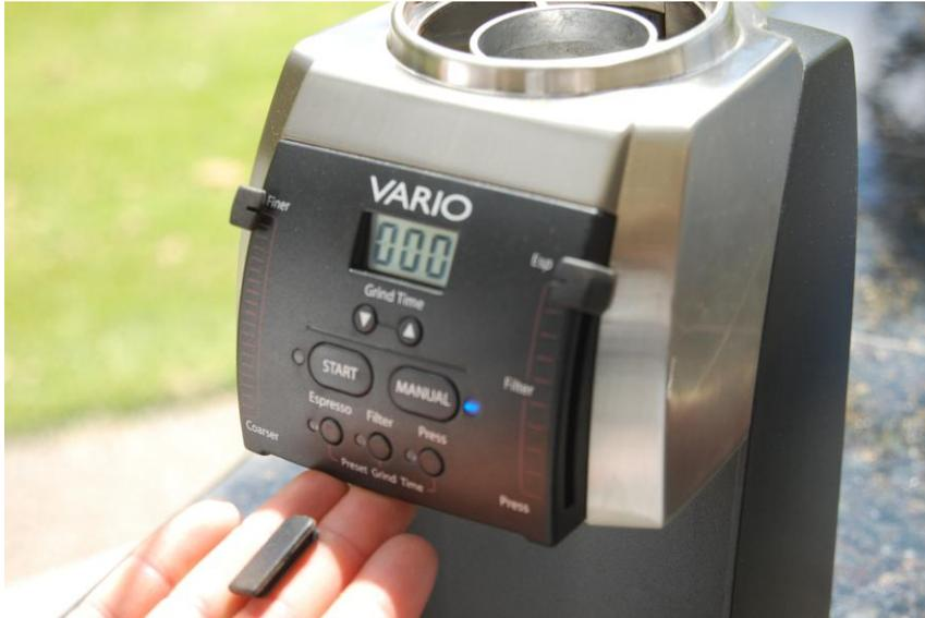
Loosen the 2mm calibration screw in the hole until it comes out. Then put it back in, only threading it one rotation.
