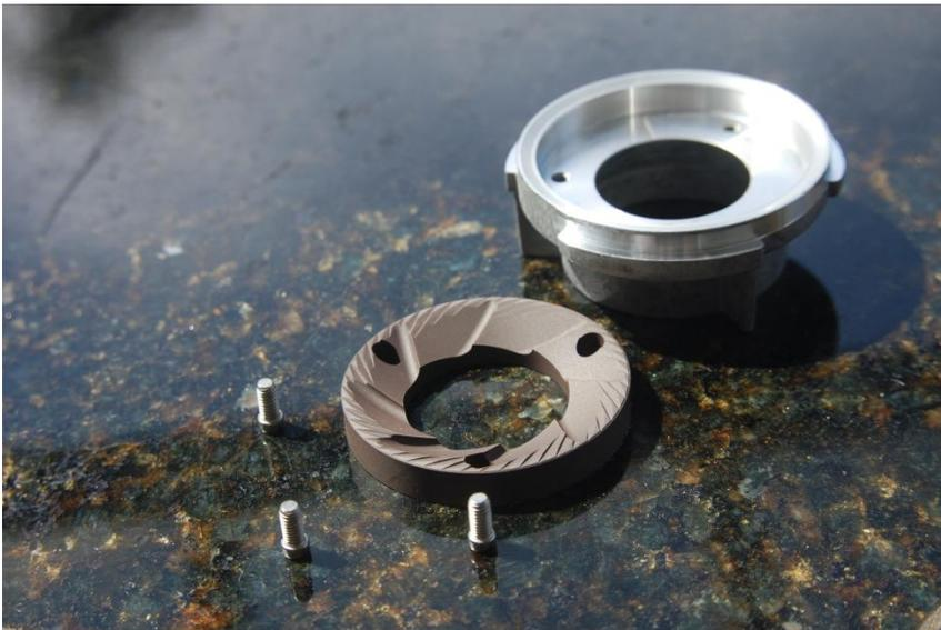
Clean the burr well. Put the burr in the new carrier, and tighten down the screws. Res assemble and test grind. You will find that the grinder does a good coarse grind, but now needs to be fine tuned for espresso. Follow the calibration guide above to accomplish this.
