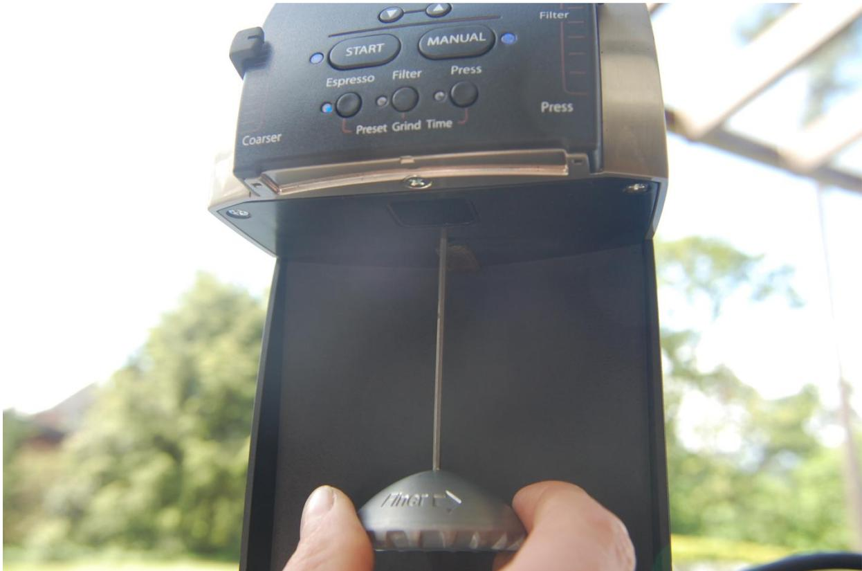
Slowly twist the tool finer until you begin to hear the motor labor and change pitch. The burrs are beginning to touch at this point.
